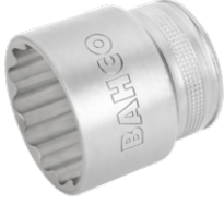
Standart lokma, 1/2" kare shaft. Çift altıgen profil, metrik 7800DM-17
